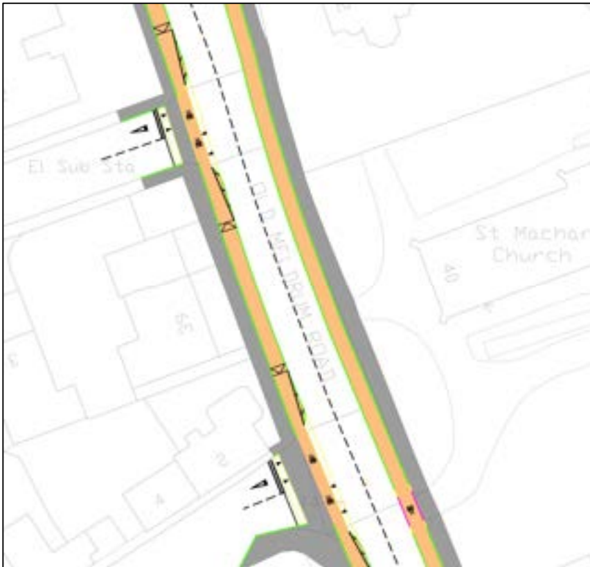
Figure 13 – Proposed with-flow cycleway arrangement
