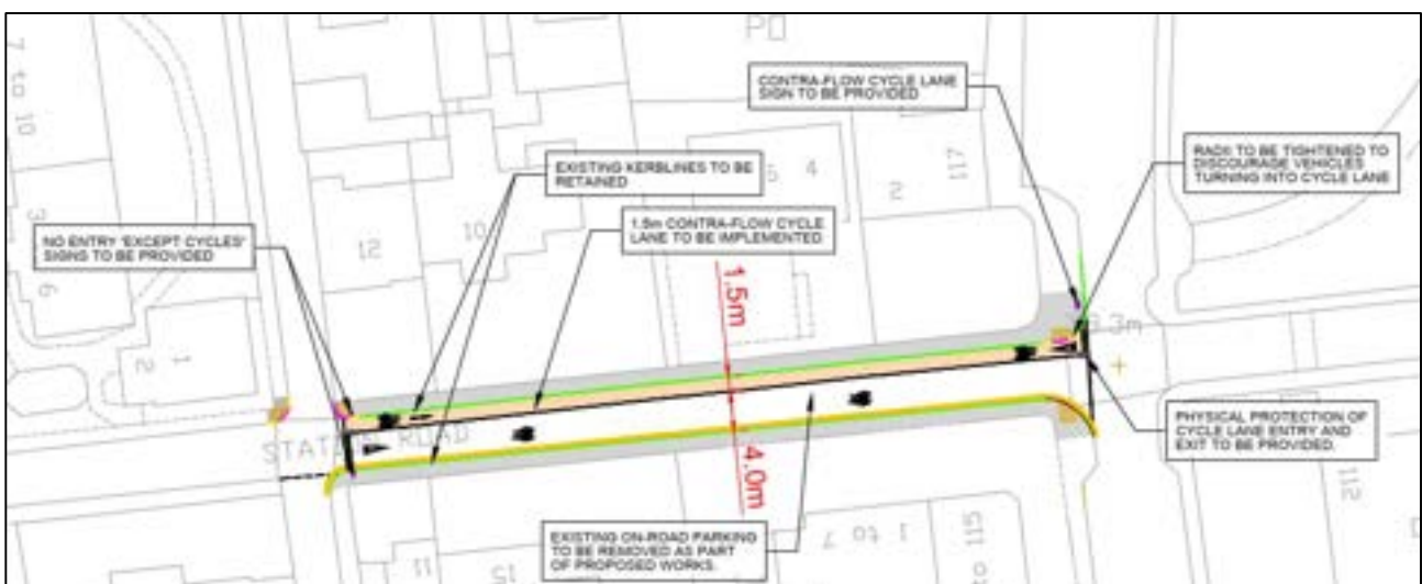
Figure 3 – Proposed layout of new segregated cycleway on Station Road
