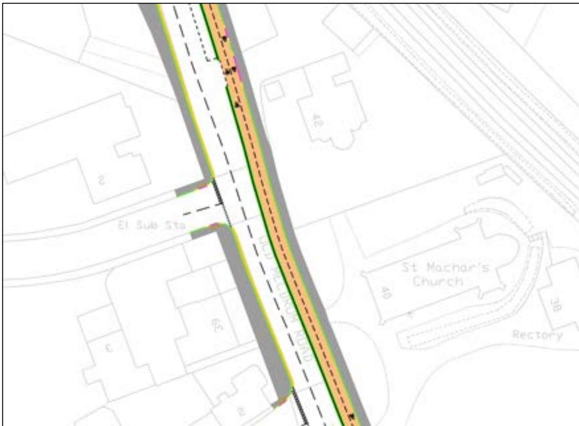
Figure 14 – Proposed two-way cycleway arrangement
