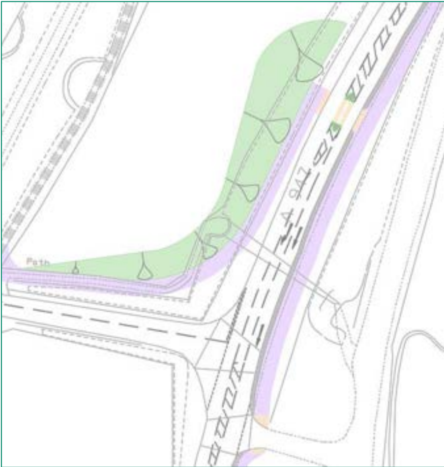
Figure 9 - Proposed Formal Crossing Arrangement to Facilitate Access to F&B Way
