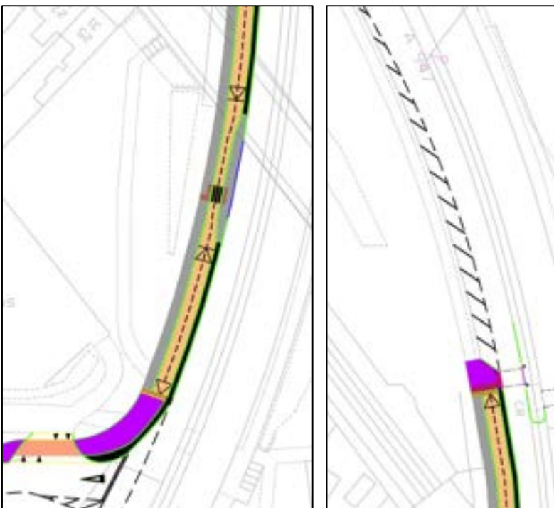
Figure 6 – Proposed segregated cycleway layout and A947 road taper
