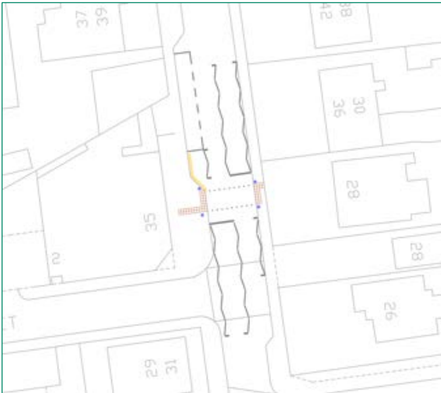
Figure 15 - New puffin crossing on Victoria Street
