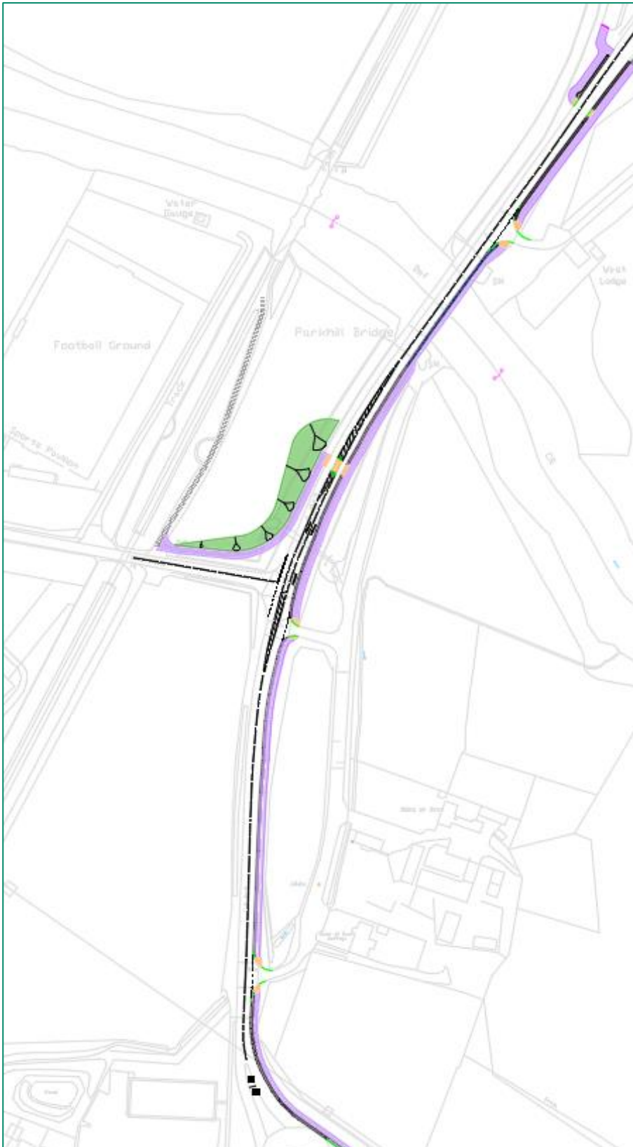
Figure 214 - Proposed extent of shared use path widening on A947 north of Riverview Drive
