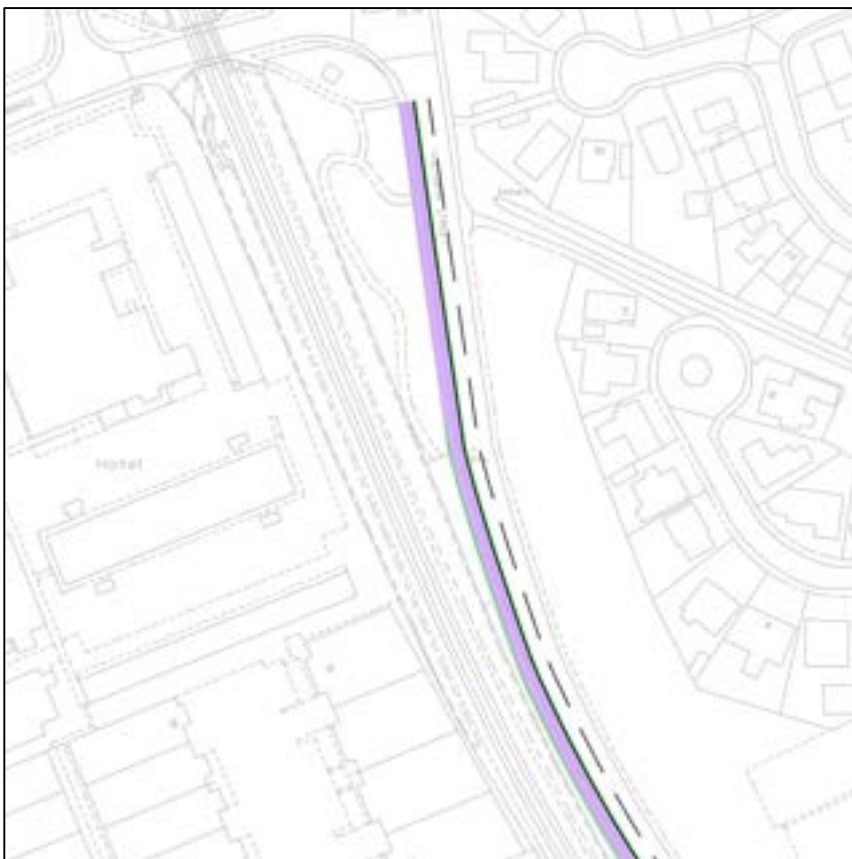
Figure 16 – Widened footways along Victoria Street south of Farburn Terrace
